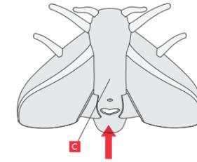
3. Attach the smoke alarm by pressing it firmly against the ceiling for approximately 30 seconds. You may also hear an alarm sound if the test button gets pressed during installation.
