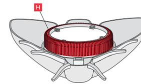
7. (Maintenance) Vacuum the smoke alarm from the grill indicated by the orange area (H) using maximum suction power.
