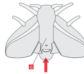
6. Make sure that the smoke alarm is activated by pressing the whole-surface test button for 3 seconds (G). When the smoke alarm gives an alarm sound, the testing has been performed successfully and your smoke alarm is ready for use. *The installation is now complete. Test your smoke alarm weekly!*
