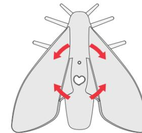
5. You can make small changes in the position of the smoke alarm by turning it a few degrees in the direction you want.
