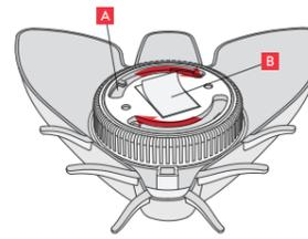
1. Activate the device by pushing the mounting plate and turning it clockwise at the same time (A). The device is activated and ready to be installed when you feel clicks. You may also hear an alarm sound if the test button gets pressed during activation.
