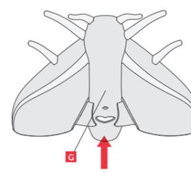
6. Make sure that the smoke alarm is activated by pressing the whole-surface test button for 3 seconds (G). When the smoke alarm gives an alarm sound, the testing has been performed successfully and your smoke alarm is ready for use. *The installation is now complete. Test your smoke alarm weekly!*
