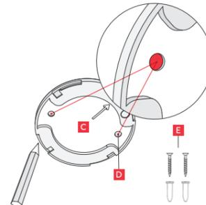
2. To achieve the correct smoke alarm positioning, you can direct your smoke alarm with the aid of the direction arrow (C) on the mounting plate. The arrow indicates the final position of the smoke alarm: square edge for Kupu and head for Lento.
